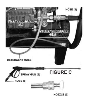
4. Attach the Hose (8) to the Spray Gun (6). Connect the other end of the Hose to the Outlet Connector (55). Connect a garden hose to the Inlet Connector (59). Insert the Detergent Hose into an approved container of detergent. Then attach the desired Nozzle (9) to the Spray Gun. (See Figure C.)
